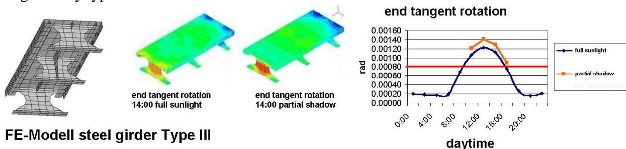
Fig. 6 Results of analysis for a double-span steel girder with variable cross section
