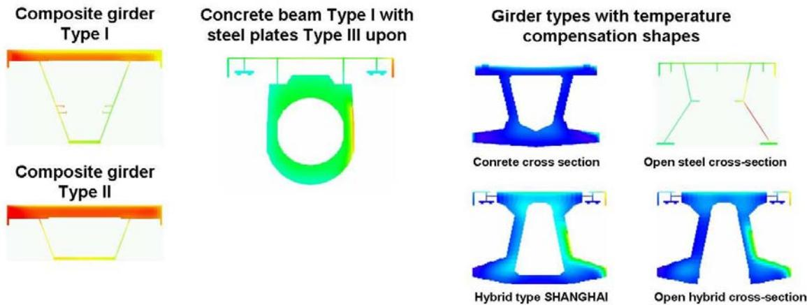
Fig. 7 Temperature distributions over alternative cross-sections
