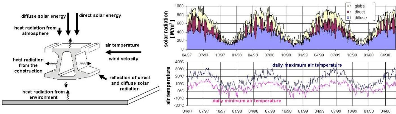
Fig. 2 Thermal environment of guideways on the testing facility in Emsland/Germany
