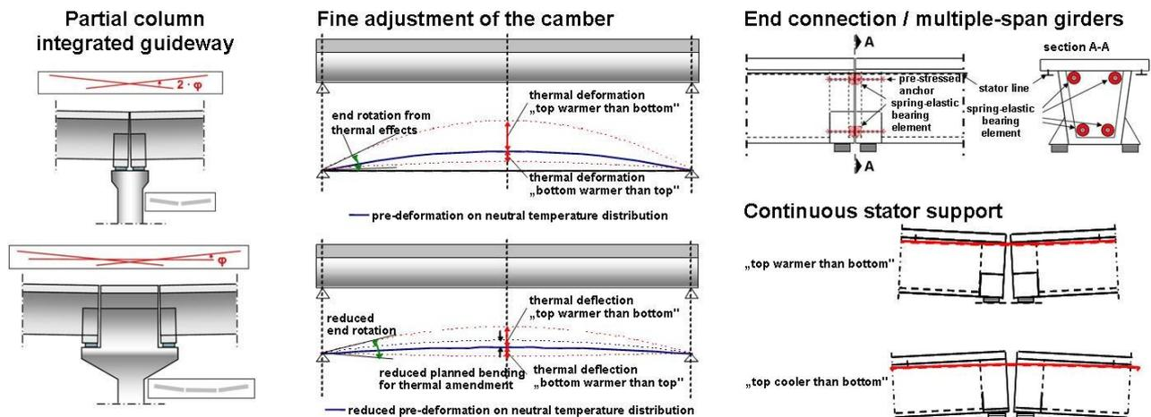
Fig. 8 Proposed modifications to the structural systems for temperature effect amendment
