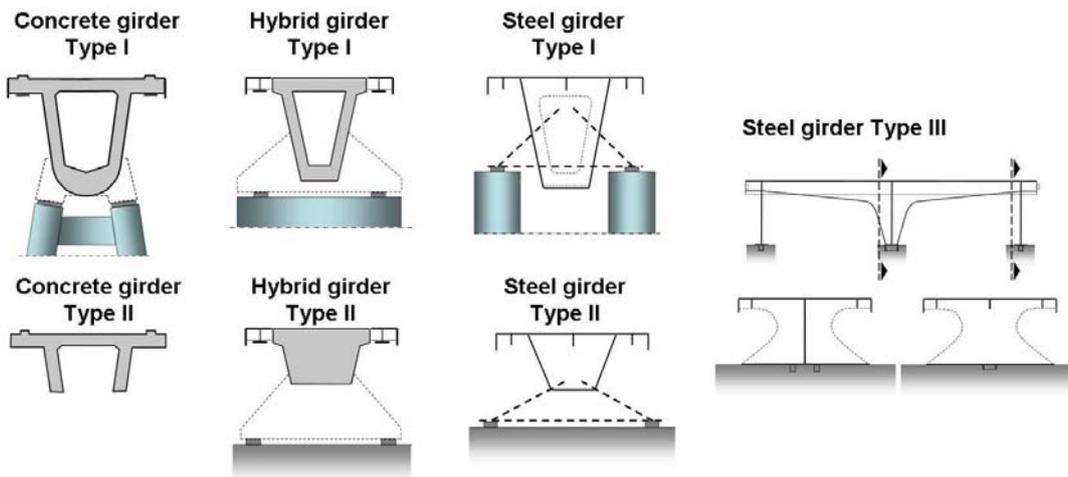
Fig. 4 Examples for analyzed existing or planned girders
