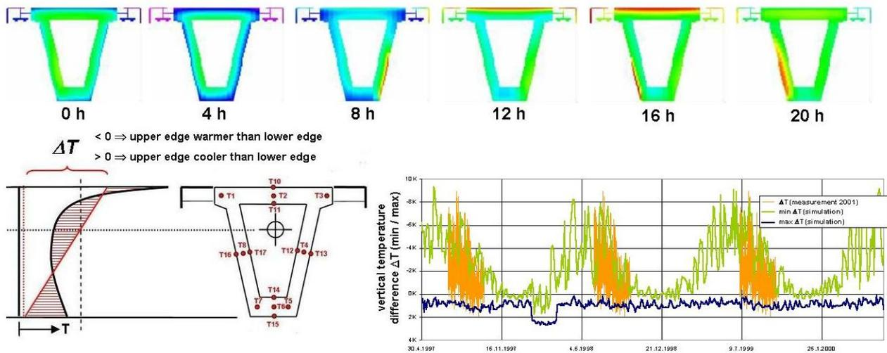
Fig. 3 Examples for calculated temperature distributions, comparison between simulation and measurement for a double-span hybrid girder on testing facility in Emsland/Germany
