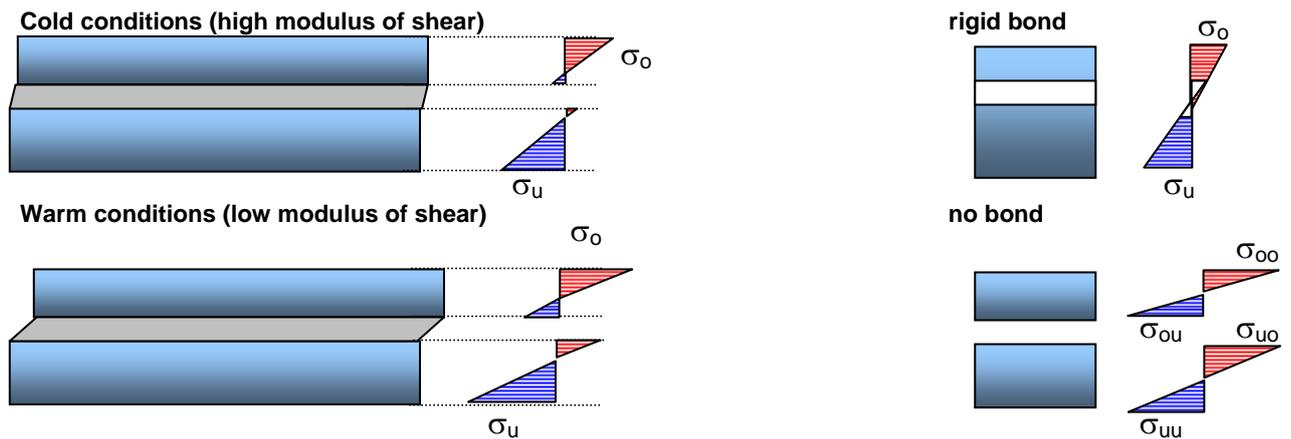
**Fig 3.** Stress distributions in different thermal conditions and long term loading
