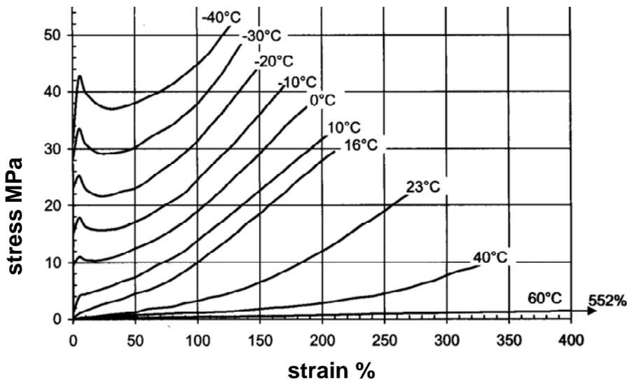
**Fig. 2** Temperature dependent strain-stress-diagram of TROSIFOL MB
