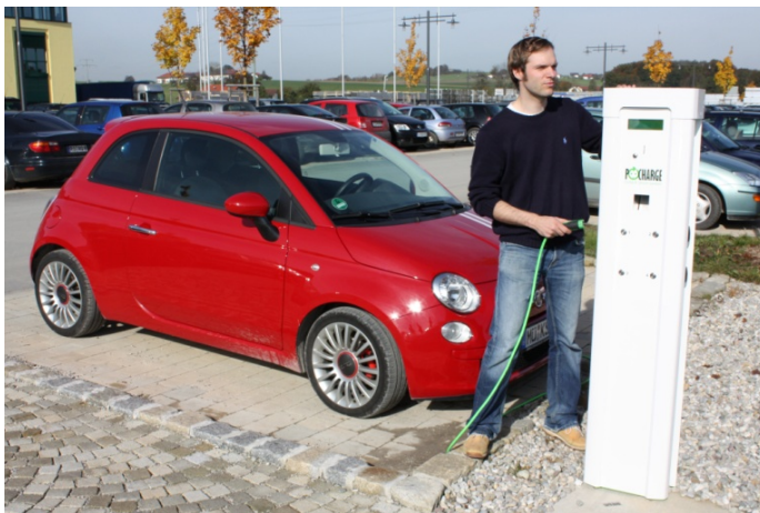
Picture 3: Charging pillar for electric vehicles
