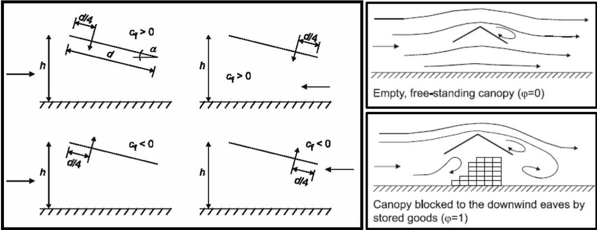
**Picture 8** Load assumptions for self-supporting roofs according to EN 1991-1-4
