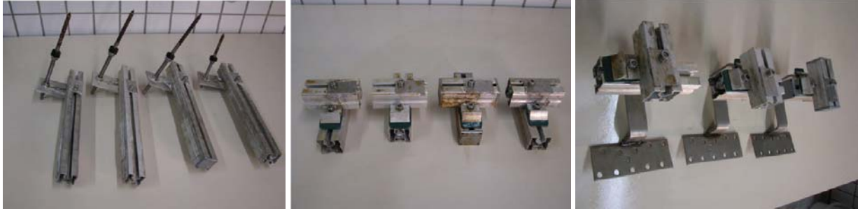
Figure 6: Test bodies with different fastening details after a successful salt spray test
